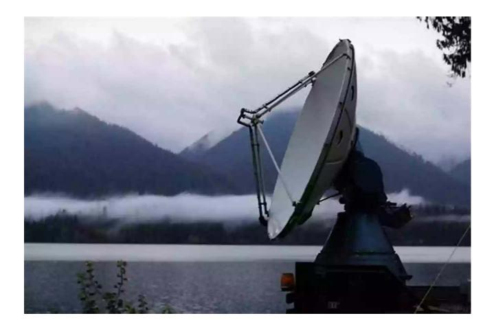
Weather radars are powerful instruments used to observe and analyze precipitation patterns in the atmosphere. By emitting radio waves that bounce off precipitation particles, weather radars can measure rainfall intensity, track the movement of rain clouds, and estimate the rate at which rain will fall in specific areas.
