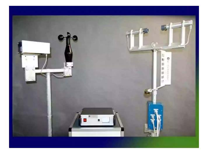
Disdrometers are scientific instruments designed to measure characteristics of raindrops, such as size and velocity, as they fall to the ground. By analyzing these characteristics, meteorologists can gain valuable insights into the intensity and volume of rain that will be experienced.
