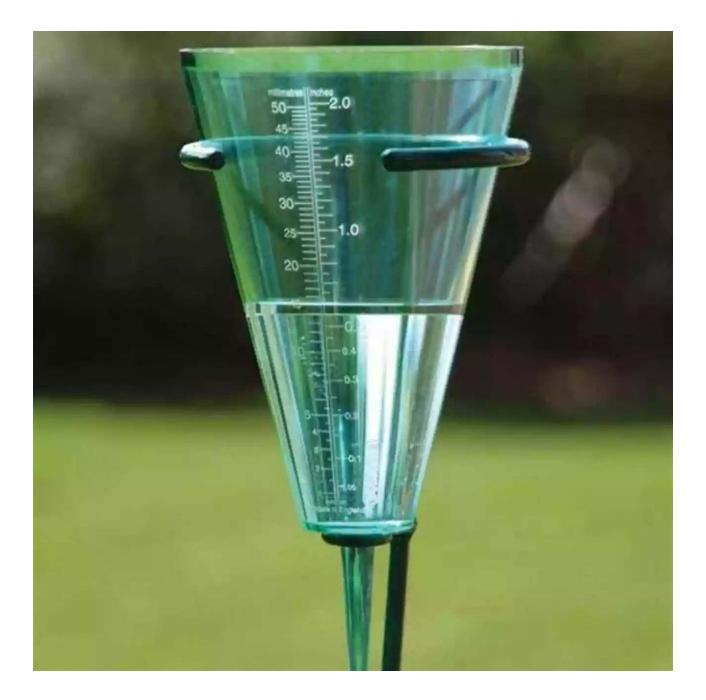
The most basic and widely recognized instrument for measuring rainfall is the rain gauge. Consisting of a cylindrical container with measurement markings, it accurately collects and measures rainwater. With modern technological enhancements, rain gauges now incorporate electronic measurement systems, enhancing data accuracy and enabling remote tracking of rainfall patterns.
