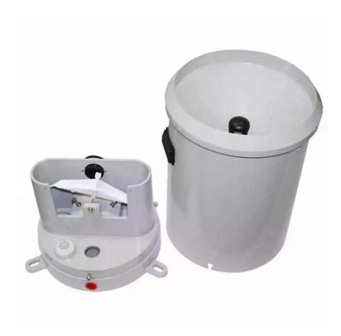
One of the advancements in rain gauges is the tipping bucket rain gauge. This automated instrument consists of a funnel that collects and channels rainwater into two compartments. With every measured amount of rainfall, the internal mechanism flips the compartments, ensuring accurate and reliable measurements. The tipping bucket rain gauge can be further enhanced with sensors that record and transmit data in real-time, enabling quick analysis and forecasting.
